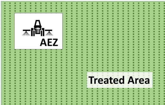
Figure 3. The AEZ is the white area around the application equipment shown above; it moves with the equipment. The AEZ generally is within the treated area, except when the application equipment is near the edges of the treated area.
